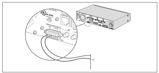
figure 4.4: Connecting 70 Volt input signal
